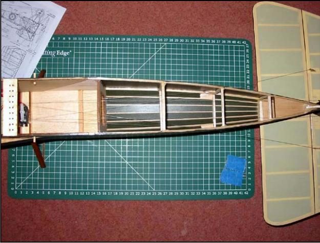
**Pull-Pull Elevator Set Up**
